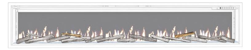
10b. Select the two mini logs and lay these on top of the first pair of slim logs.
