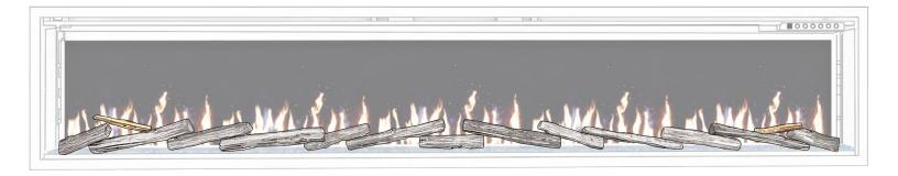
9b. Select two mini logs and lay these on top of the second pair of slim logs.
