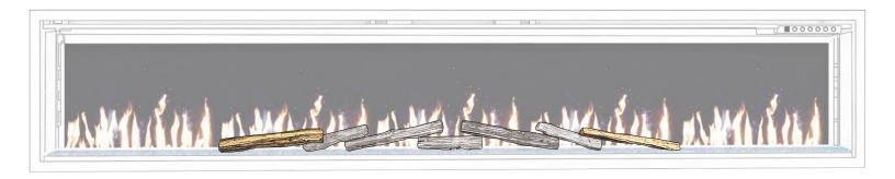
5. Select two slim logs, and stack these on the ends of the slim logs.
