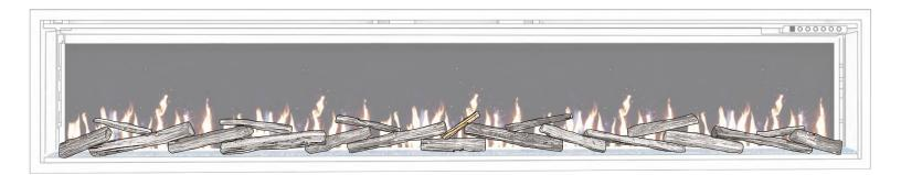
12b. Use the bag of wood chips and place a few chips and chunks in the gaps between the logs. We recommend using these sparingly for the best appearance and to maximize the light output from the ember bed.
