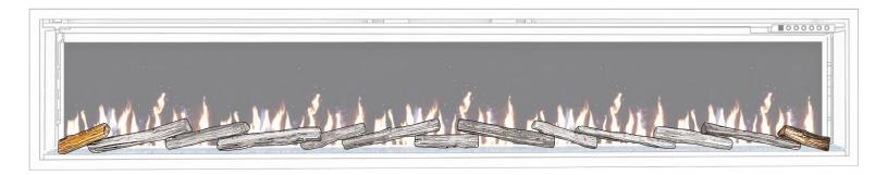
8b. Select two mini logs and lay these on top of the slim logs previously stacked. Note that adding the mini logs is optional.
